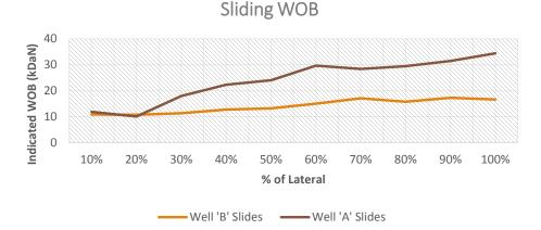
This chart plots the average WOB in 10% increments along the lateral sections of each well. It can be seen that Well "A" experienced a dramatic increase in WOB indicated at surface. This would be consistent with significantly increased drag as the well progressed deeper and deeper. It should also be noted that the Ratler prevented significant drag increases through the progression of Well "B" allowing it to experience continued ROP gains over the other well.
