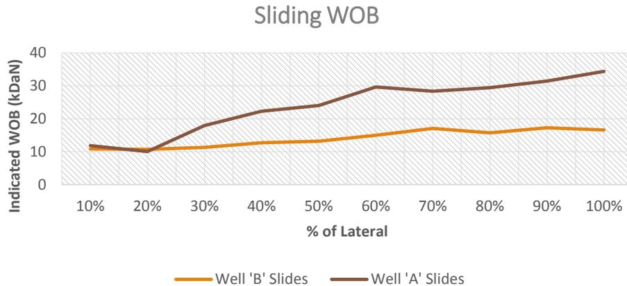
This chart plots the average WOB in 10% increments along the lateral sections of each well. It can be seen that Well "A" experienced a dramatic increase in WOB indicated at surface. This would be consistent with significantly increased drag as the well progressed deeper and deeper. It should also be noted that the Ratler prevented significant drag increases through the progression of Well "B" allowing it to experience continued ROP gains over the other well.
