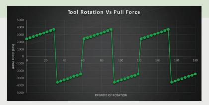
Theoretical axial force generated with tool through 180 degrees of rotation. (This assumes 20% ecency due to slippage and formation integrity)
